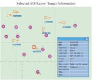
Through receiving the data of sensor, such as GPS, heading sensor, 3G module etc, display the position, course, speed etc. of the ship in real time. It is able to indicate the status of the external sensor with different color.
